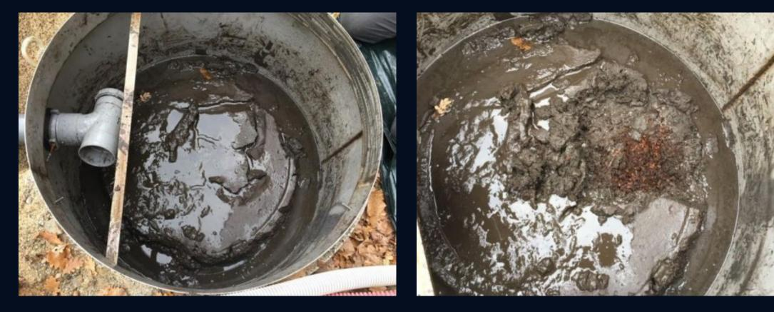
Filter – Downstream of 2-days HRT SBR system treating 1,260 L/d for six months
