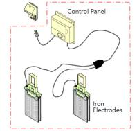
Fig. 2 Phosphorus removal device
