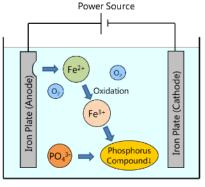
Fig. 3 Process of phosphorus removal
