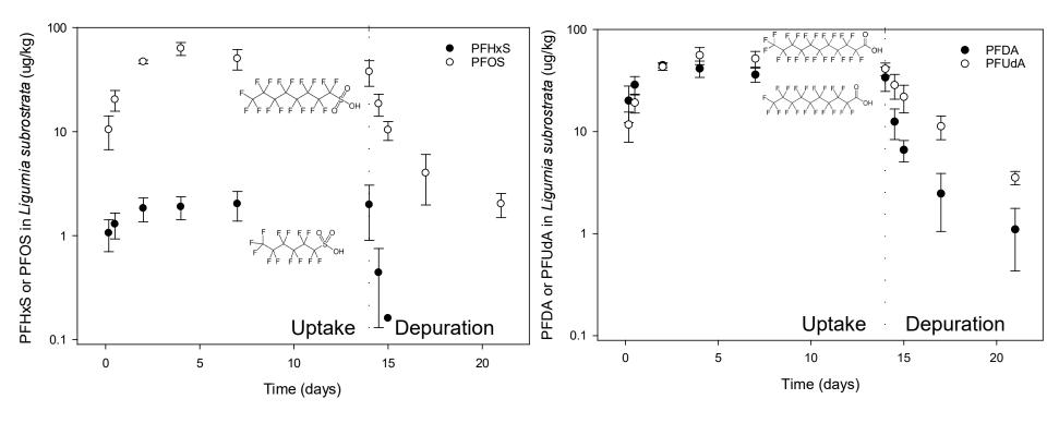
Uptake and elimination of A. PFHxS and PFOS, and B. PFDA and PFUdA by the freshwater pond mussel, *Ligurnia subrostrata*. A 14 day uptake period occurred with exposure to PFHxS, PFOS, and PFDA at 10  $\mu$ g/L and PFUdA at 1  $\mu$ g/L. The vertical reference line denotes when a seven day elimination period was initiated.
