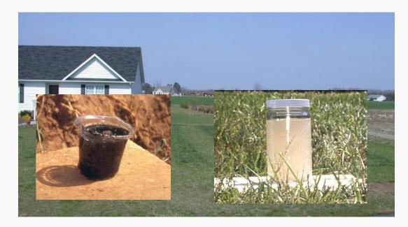
Primary treatment by a septic tank (~20%), rest (~80%) by soil. Aerobic tank spray-field
