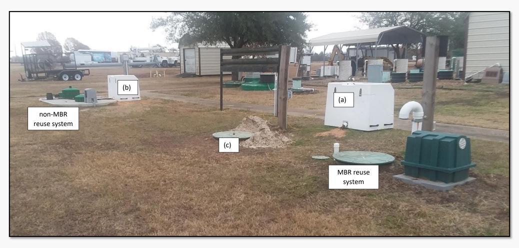
(a) and (b) are the weather-proof boxes each housing two refrigerated composite samplers. (c) is ozone tank for MBR effluent.
