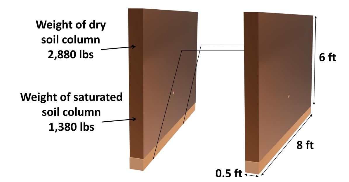
3-D View of Anchor Ballasts and Overlying Soil Columns
