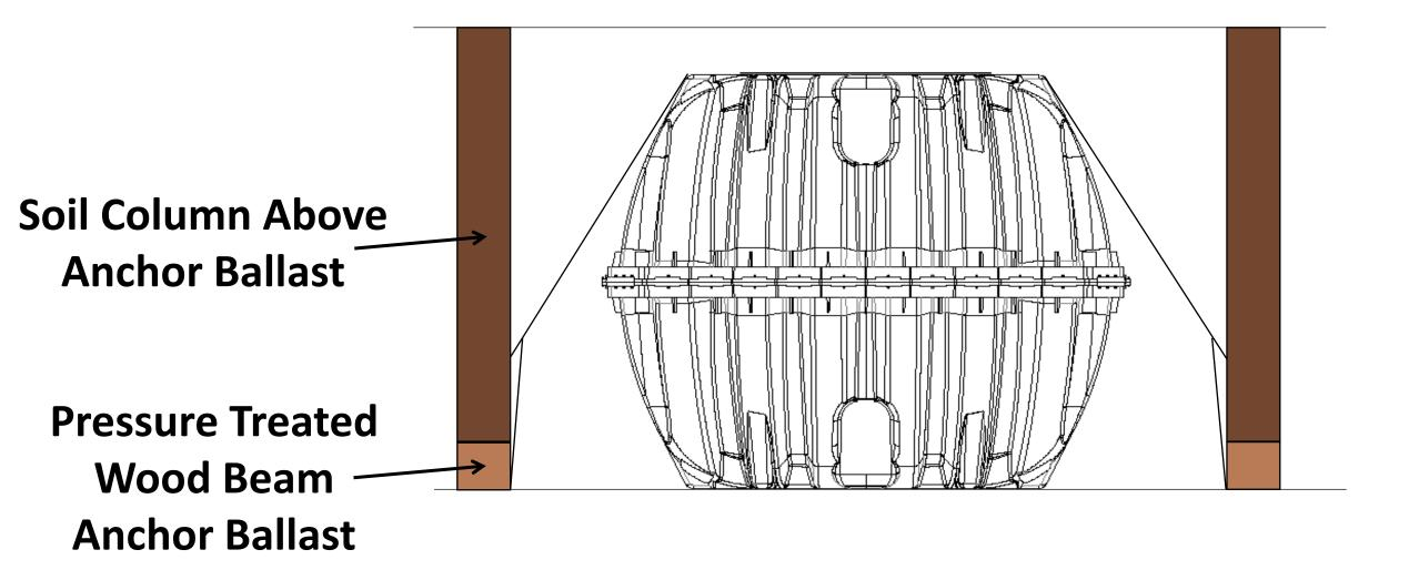
3-D View of Anchor Ballasts and Overlying Soil Columns
