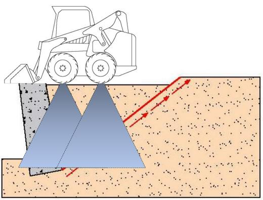
Will the skid steer load move the wall or retained soil?
