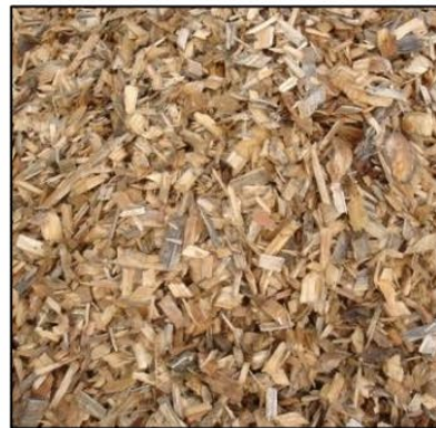
denitrification media: lignocellulosics & elemental sulfur
