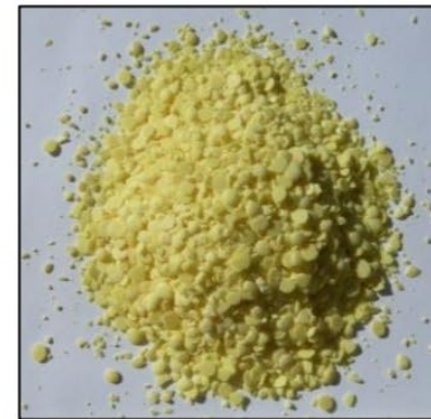
denitrification media: lignocellulosics & elemental sulfur
