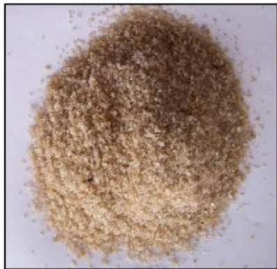
nitrification media: sand & expanded clay
