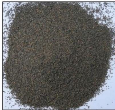
nitrification media: sand & expanded clay
