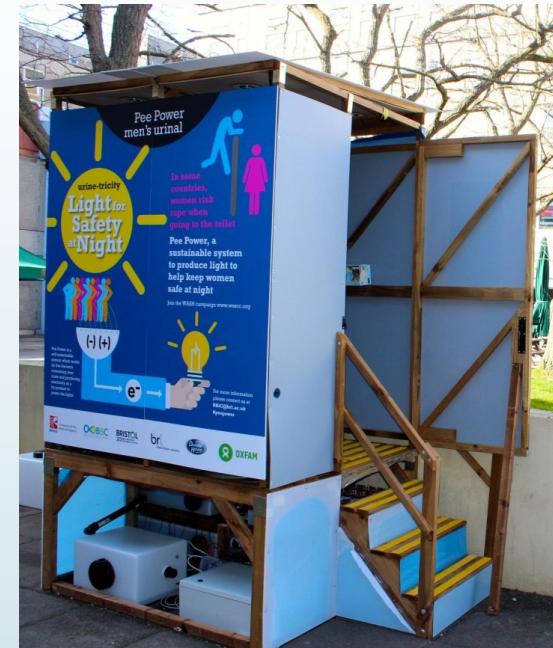
V1. Pee Power toilet with stack of MFCs underneath. Lights of the toilet were powered
