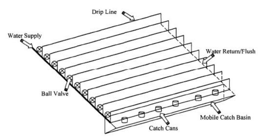
Figure 4. Emitter testing layout (Duan, 2006<sup>6</sup>)
