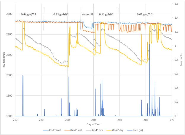
Figure 1 Results from the 4-inch depth soil moisture sensors. The Day of Year is for 2021, DOY 210 is July 29. As shown in this graph, the soil moisture content is represented by the millivolt output of the sensors, higher millivolt readings indicate greater soil moisture content.
