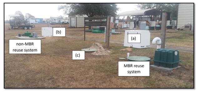
Figure 6: Field layout of the MBR and non-MBR reuse systems. (a) and (b) are the weather-proof boxes each housing two refrigerated composite samplers. (c) is ozone tank for MBR effluent.
