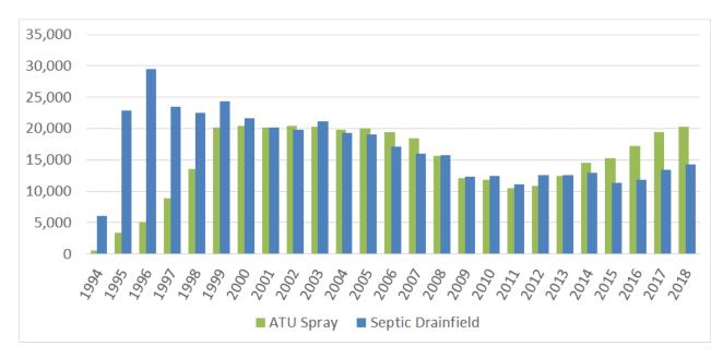
Figure 2: Trend showing increasing use of ATU (*Aerobic Treatment Unit*) Spray in Texas since mid-1990s. Y-axis shows the number of permits issued in Texas and X-axis is the Year.
