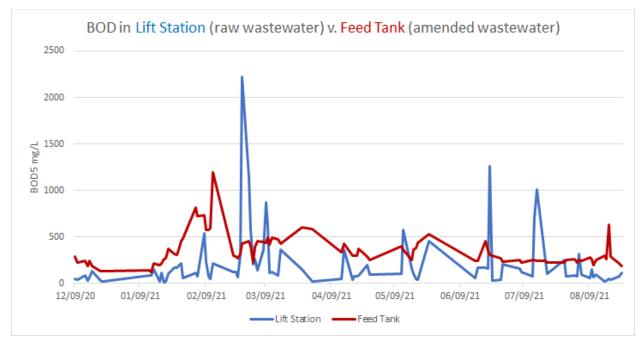
Figure 7: Effects of amending raw wastewater by daily addition of MAF in feed tank effluent BOD5. Similar effects were observed for TSS also.
