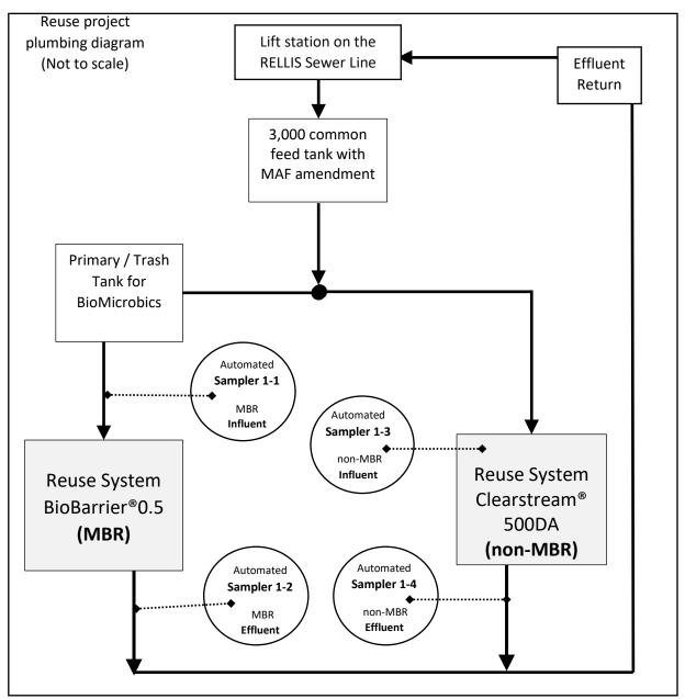
Figure 5: Flow path for the Reuse project. Note that the influent to both the reuse technologies was the same, however the daily flow rate varies due to the configuration of influent pipe.
