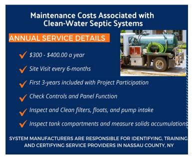
Figure 3: Operation and Maintenance Requirements
