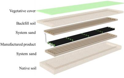
Fig. 1 – Exploded view of typical CTD components
