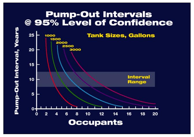
The pumping interval for properly sized and managed watertight tanks is about 12-20 years.
