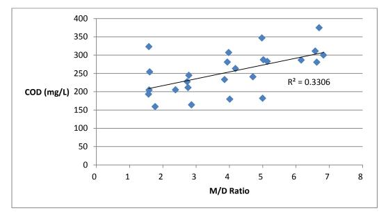
Figure 4-4. R<sup>2</sup> Correlation of M/D Ratio and COD Measurements of Column Effluent of the Final Five Complete Measurements of the First Run (Determining the Effect of Water Softener Usage on Septic Tank Effluent)
