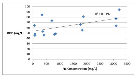
Figure 4-40. BOD versus Sodium Concentration For the Fifth Run (Duplicate Study Determining the Effect of Regeneration Wastes With Greater Sodium Concentrations on Septic Tank Effluent)
