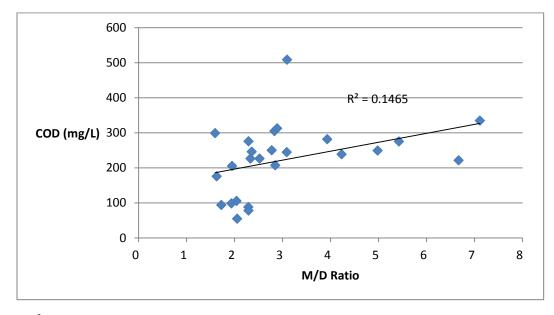
Figure 4-13. R<sup>2</sup> Correlation of M/D Ratio and COD Measurements of Column Effluent of Final Five Complete Measurements of the Second Run (Determining the Effect of Regeneration Wastes on Septic Tank Effluent)
