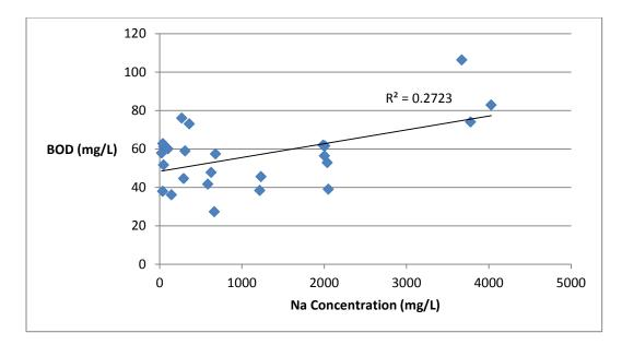
Figure 4-30. Correlation of Sodium Concentration and BOD<sub>5</sub> Measurements of Column Effluent of Final Five Complete Measurements of the Fourth Run (Determining the Effect of Regeneration Wastes With Greater Sodium Concentrations on Septic Tank Effluent)
