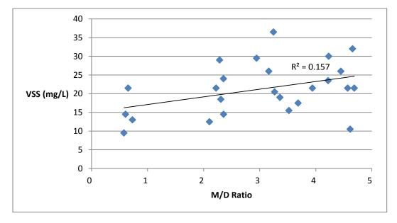
Figure 4-20. Correlation of M/D Ratio and VSS Measurements of Column Effluent of Final Five Complete Measurements of the Third Run (Determining the Effect of Sodium in Regeneration Wastes on Septic Tank Effluent)
