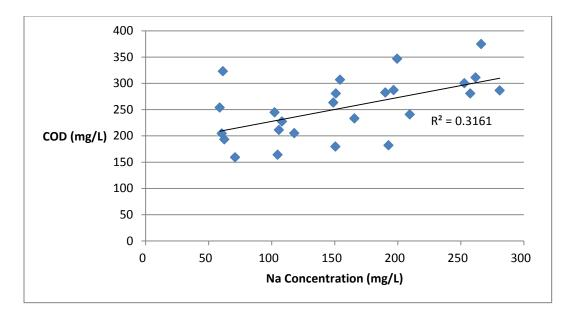
Figure 4-5. R<sup>2</sup> Correlation of Sodium Concentration and COD Measurements of Column Effluent of the Final Five Complete Measurements of the First Run (Determining the Effect of Water Softener Usage on Septic Tank Effluent)
