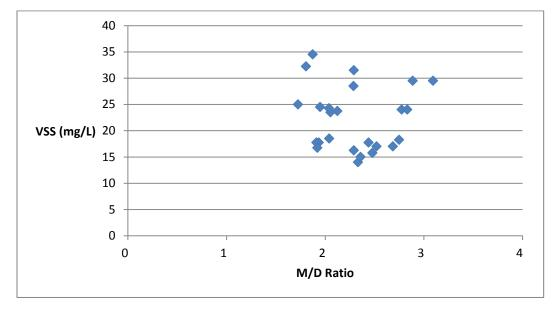
Figure 4-15. R<sup>2</sup> Correlation of M/D Ratio and VSS Measurements of Column Effluent of Final Five Complete Measurements of the Second Run (Determining the Effect of Regeneration Wastes on Septic Tank Effluent)
