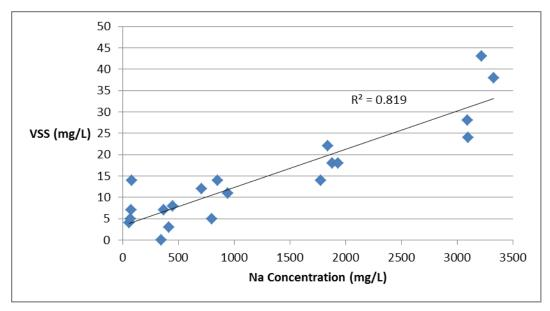
Figure 4-39. VSS versus Sodium Concentration For the Fifth Run (Duplicate Study Determining the Effect of Regeneration Wastes With Greater Sodium Concentrations on Septic Tank Effluent)
