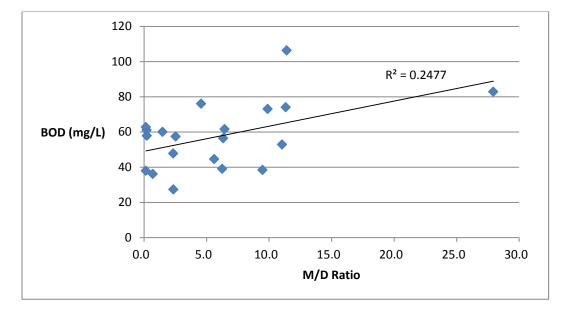
Figure 4-29. Correlation of M/D Ratio and BOD₅ Measurements of Column Effluent of Final Five Complete Measurements of the Fourth Run (Determining the Effect of Regeneration Wastes With Greater Sodium Concentrations on Septic Tank Effluent)
