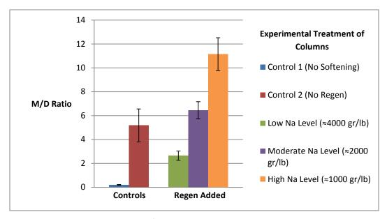
Figure 4-32. Final Five Day Average of M/D Ratio of Column Effluent During the Fifth Run (Duplicate Study Determining the Effect of Regeneration Wastes With Greater Sodium Concentrations on Septic Tank Effluent)
