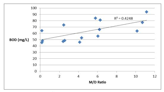
Figure 4-38. BOD versus M/D Ratio For the Fifth Run (Duplicate Study Determining the Effect of Regeneration Wastes With Greater Sodium Concentrations on Septic Tank Effluent)
