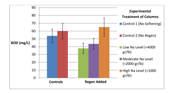
Figure 4-26. Final Five BOD₅ Measurements of Column Effluent During the Fourth Run (Determining the Effect of Regeneration Wastes With Greater Sodium Concentrations on Septic Tank Effluent) Averaged with Standard Deviations
