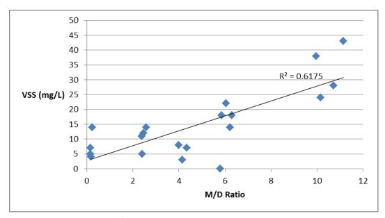
Figure 4-37. VSS versus M/D Ratio For the Fifth Run (Duplicate Study Determining the Effect of Regeneration Wastes With Greater Sodium Concentrations on Septic Tank Effluent)
