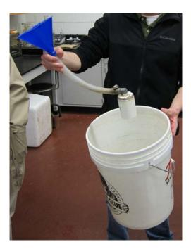
Figure 3-2. Effluent screen set up.
