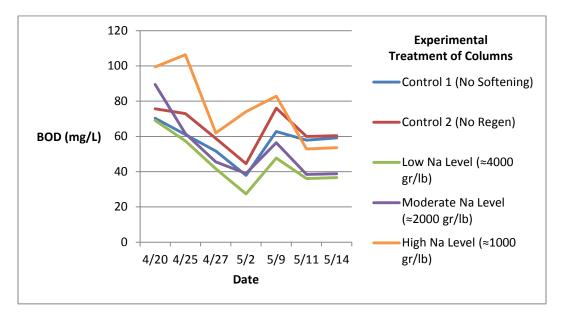
Figure 4-25. Effluent BOD₅ for the Entire Fourth Run (Determining the Effect of Regeneration Wastes With Greater Sodium Concentrations on Septic Tank Effluent)
