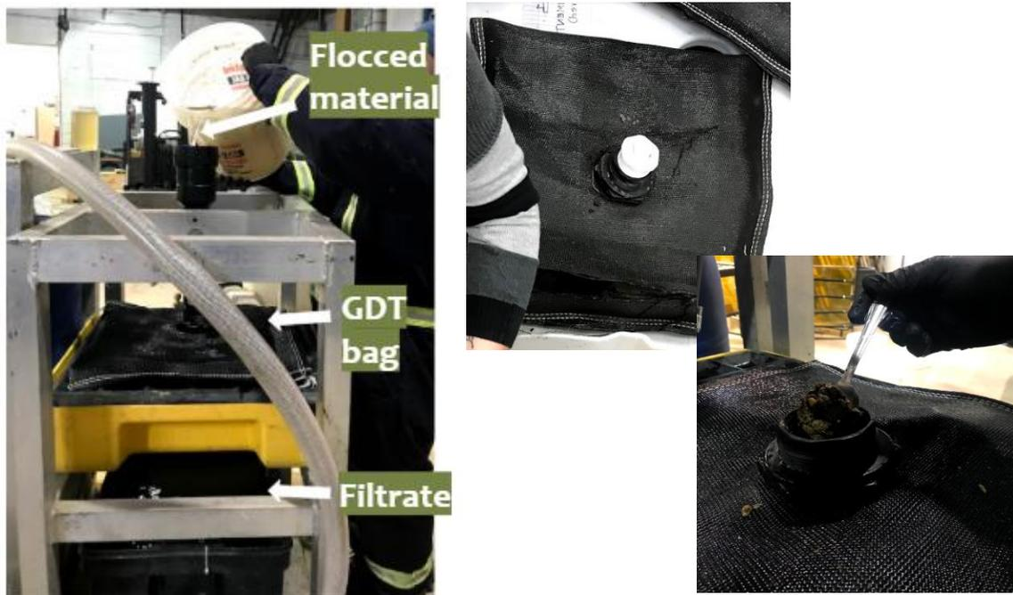
**Figure 2** Left: GDT experimental setup. Right: Storage and sampling of cakes from the GDT.
