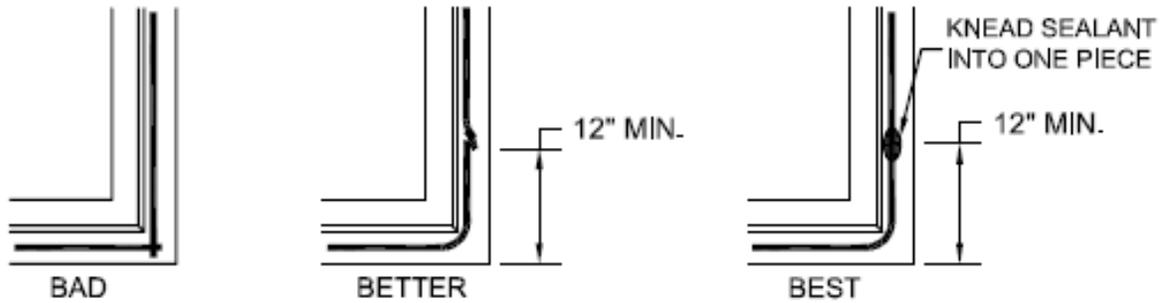
Figure 4 – Best Practices on Connecting Sealant (Courtesy of Concrete Sealants Inc.)
