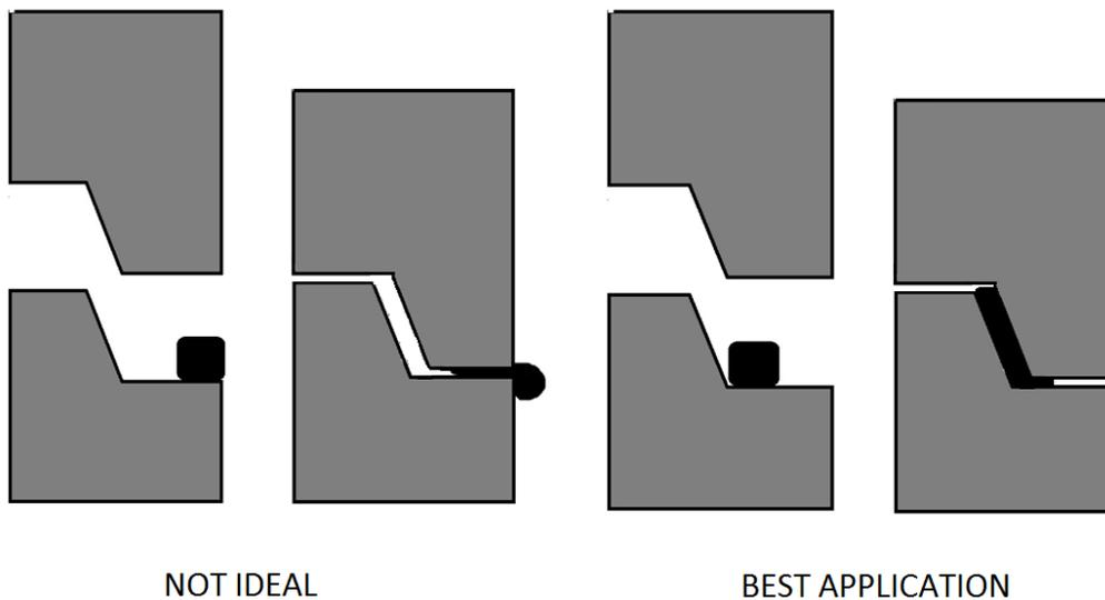
Figure 5 – Best Practices on Applying Sealant Closer to Middle of Tank Wall (Courtesy of National Precast Concrete Association)
