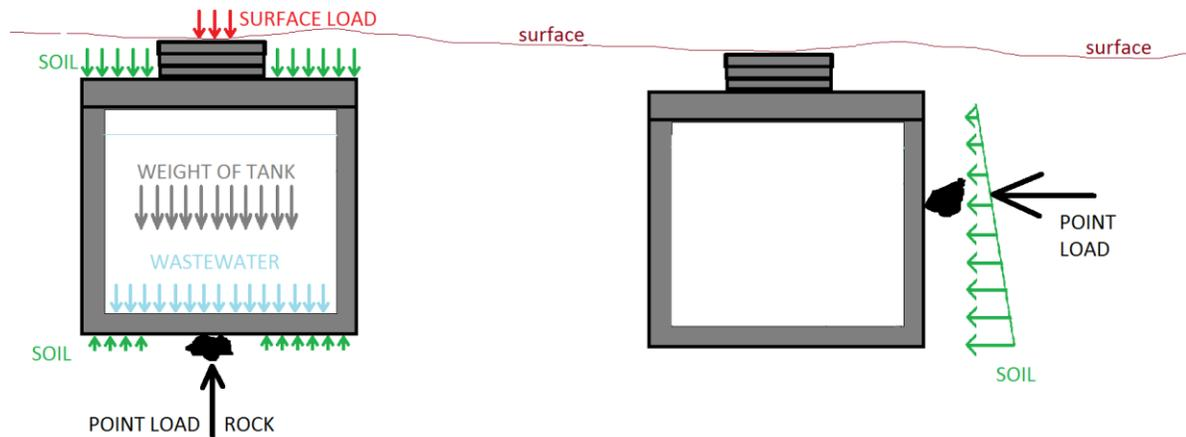
Figure 6: Illustration of Point Loads on an Underground Tank (Courtesy of National Precast Concrete Association)
