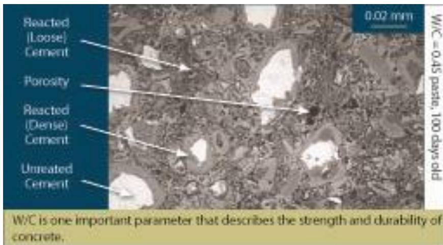
Figure 1 – Scanning Electron Microscope Image Showing Cement Paste Components and Paste Porosity (Courtesy of National precast Concrete Association)
