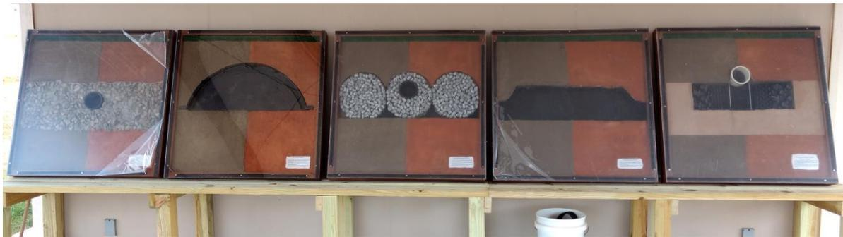
Figure 5. a) A sample shadowbox built to demonstrate the pipe and gravel distribution system. The boxes are 36 inches wide to demonstrate a trench and there are two different soils representing a North Georgia soil (Right) and a South Georgia soil (Left); b) Plexiglass covers the boxes to provide a surface to draw on for explaining various concepts of the distribution system; c) the five shadowboxes as they are displayed for educational purposes. (Images by G. Hawkins and J. Rolando Orellana).
