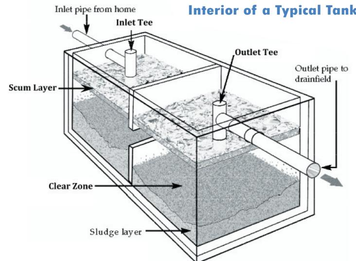
the tank where it is retained for a day or more. During the time it is in the tank, the heavier solids settle to the bottom to form a sludge layer. The lighter solids, greases and oils float to the top to form a scum layer.
