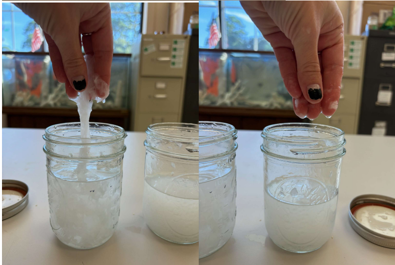
Fig. 8. The top image shows the materials needed for this model/demonstration, facial tissue, toilet paper, and jars with water and lids. After 30sec agitation, you can see the results with the facial tissue (left) is still intact and toilet paper (right) is broken down into tiny pieces. (Photos by MC Halbrook)
