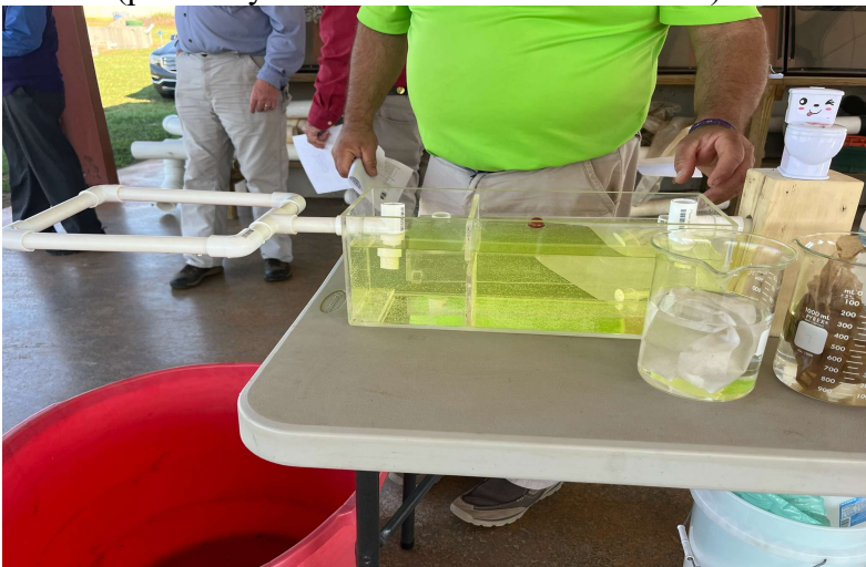
Fig. 7. Model septic system. Includes toy toilet on far right then progresses to the left. (photo by MC Halbrook)
