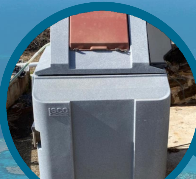
Influent Sampler: ISCO 5800 (Refrigerated)
