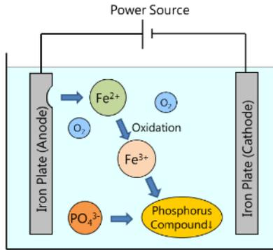
Fig. 3 Process of phosphorus removal
