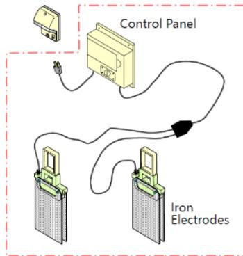
Fig. 2 Phosphorus removal device
