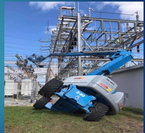
Construction lift fallen into an unmarked septic tank.
