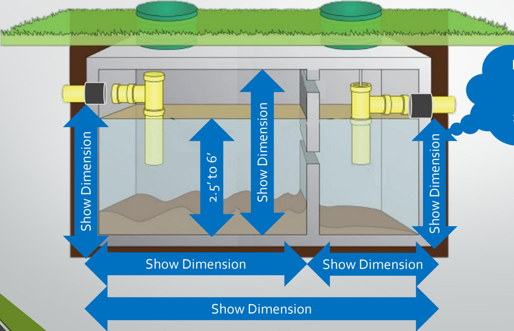
Inlet / Outlet height differential; 2" minimum
