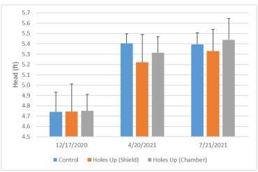
Figure 11. Pressure on laterals as measured at the beginning of the experiment (December 17, 2020), and on April 20 and July 21, 2021. Columns show the average value for each configuration, while error bars indicate the standard deviation value
