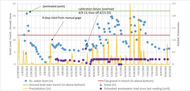
Figure 10. Average water level measured from all 24 inspection ports, daily totals of rainfall events measured at the manual rain gauge, estimated wastewater daily load, and bottom and top levels for the average trench (top indicating either gravel or chamber)
