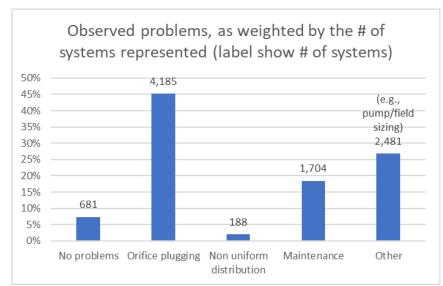
Figure 3 – Summary results from the LPD survey response. Results were weighted based on the number of OSSF designed/installed/maintained/inspected (count is reported on top of each bar)
