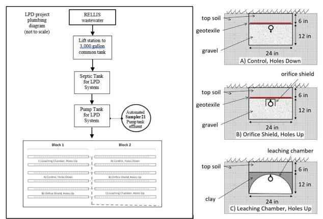
Figure 4. LPD experiment plumbing design (left), and cross-section view for three LPD Configurations (right)
