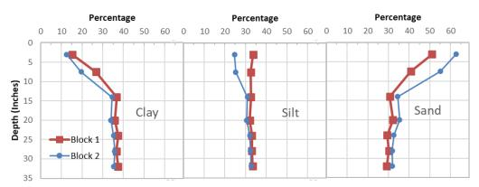
Figure 14. Soil texture observed at the South-West side (Block 1) and the North-East side (Block 2) of the LPD drain field, near the corresponding TDR sensors
