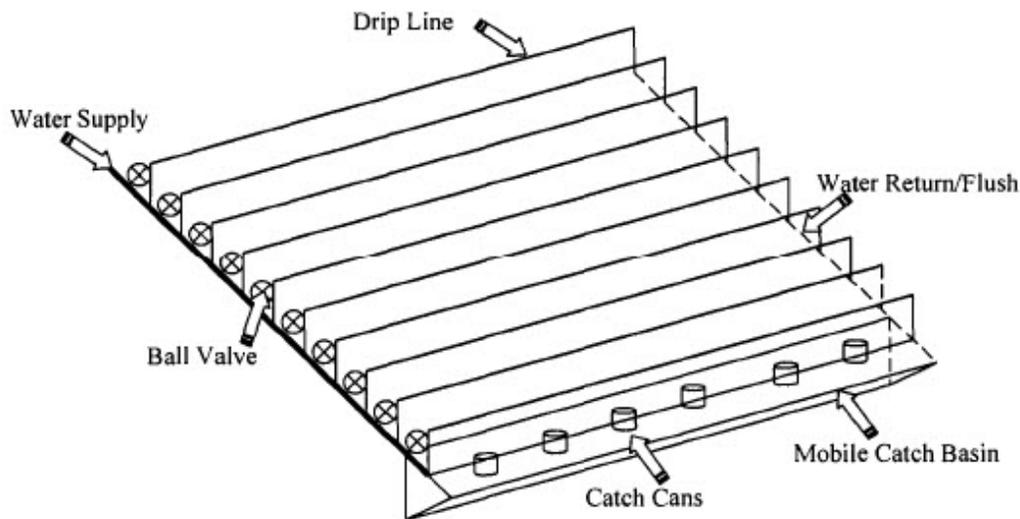
Figure 4. Emitter testing layout (Duan, 2006<sup>6</sup>)
