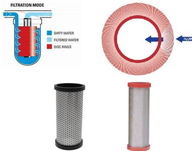
Figure 3. Disc (top) and screen (bottom) filters
