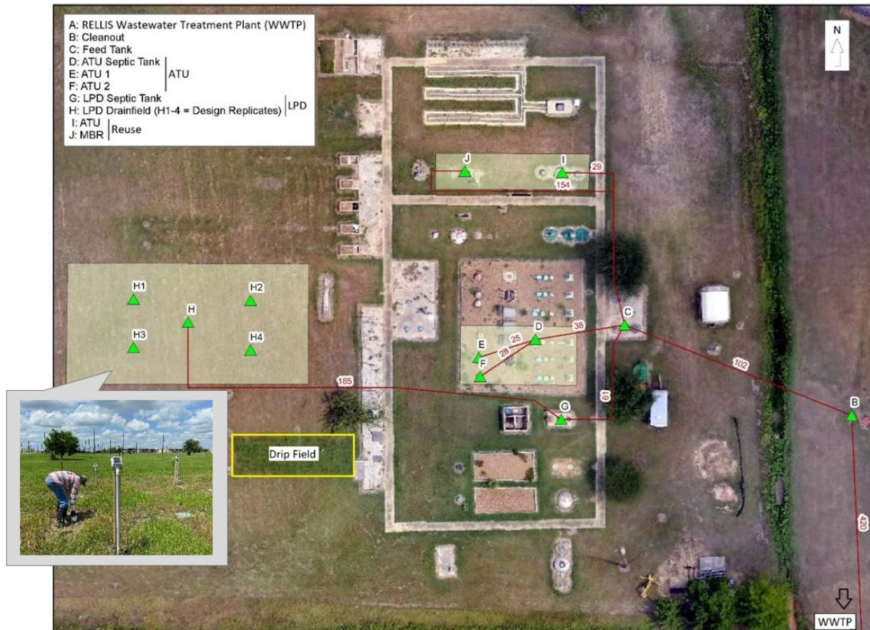
Figure 5. Aerial view of the Texas A&M RELLIS Campus, Bryan Texas, OSSF center (TAMU OSSF center). The callout shows the new Low-Pressure Dosing (LPD) drain field built within the RFGA 1st cycle, 2019
