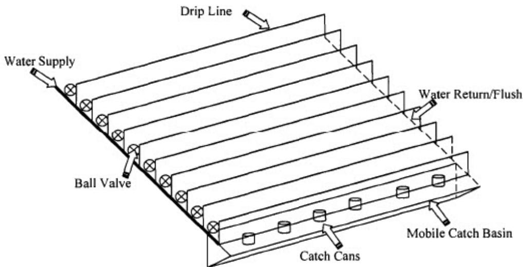
Figure 4. Emitter testing layout (Duan, 2006<sup>6</sup>)
