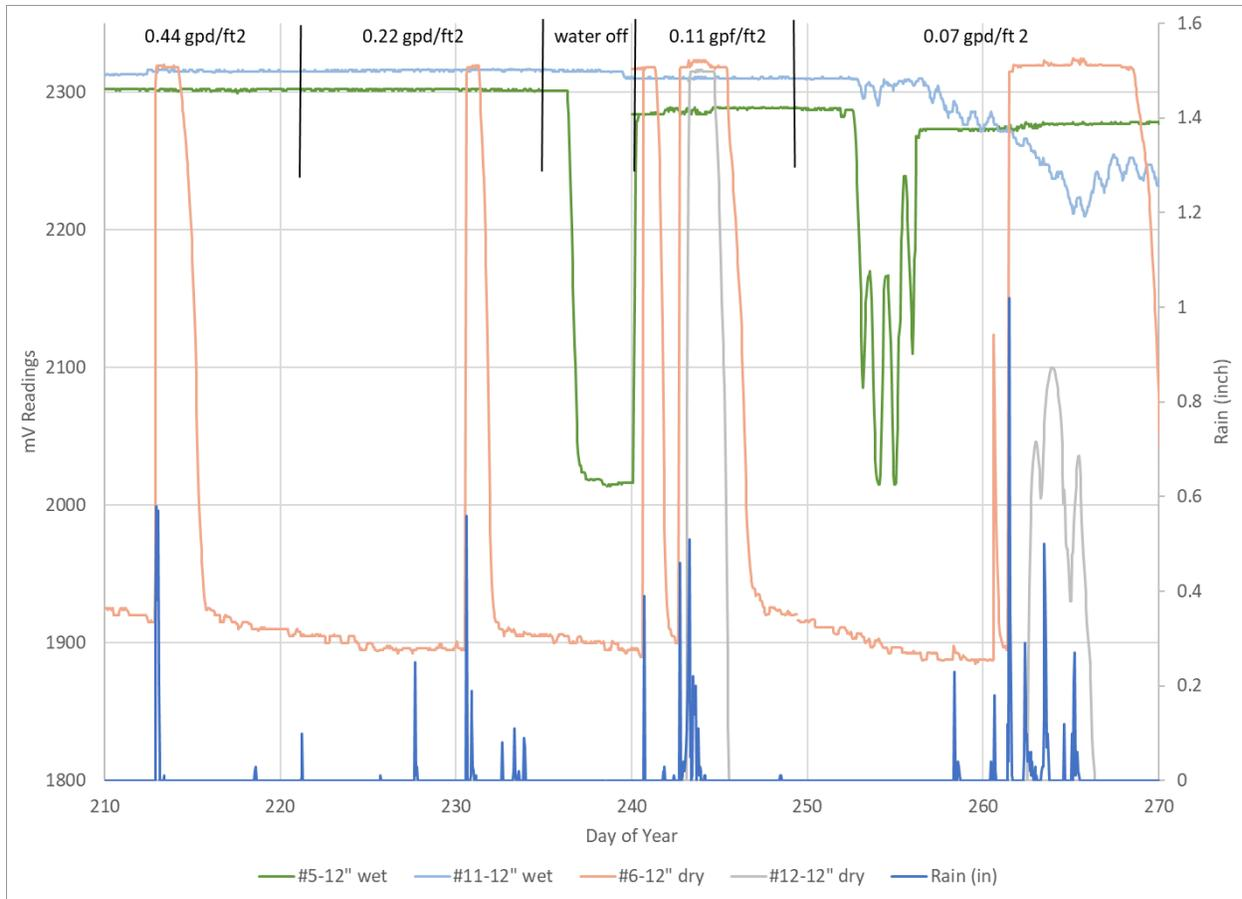
Figure 3. Results from the 12-inch depth soil moisture sensors. The Day of Year is for 2021, DOY 210 is July 29.
