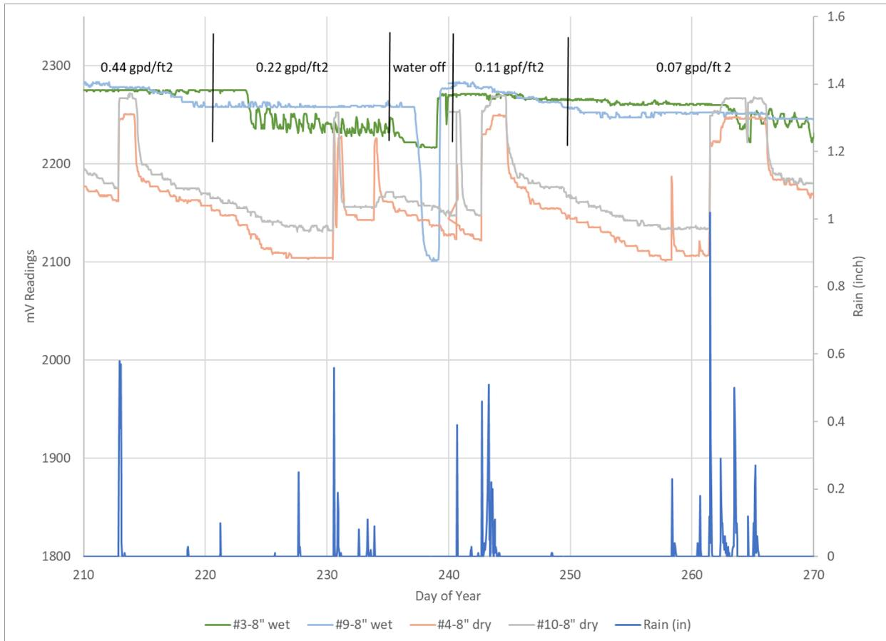
Figure 2. Results from the 8-inch depth soil moisture sensors. The Day of Year is for 2021, DOY 210 is July 29.
