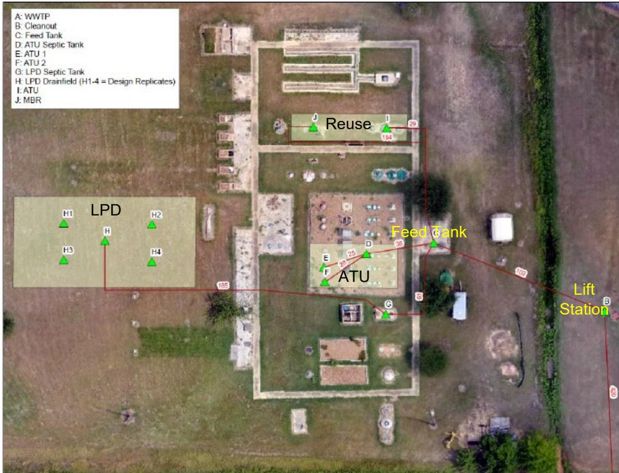
Figure 4: Aerial view of the three research project areas showing the ATU, LPD and Reuse project locations at the TAMU’s OSSF Center on RELLIS Campus.
