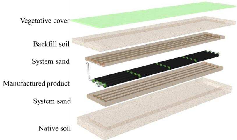
Fig. 1 – Exploded view of typical CTD components
