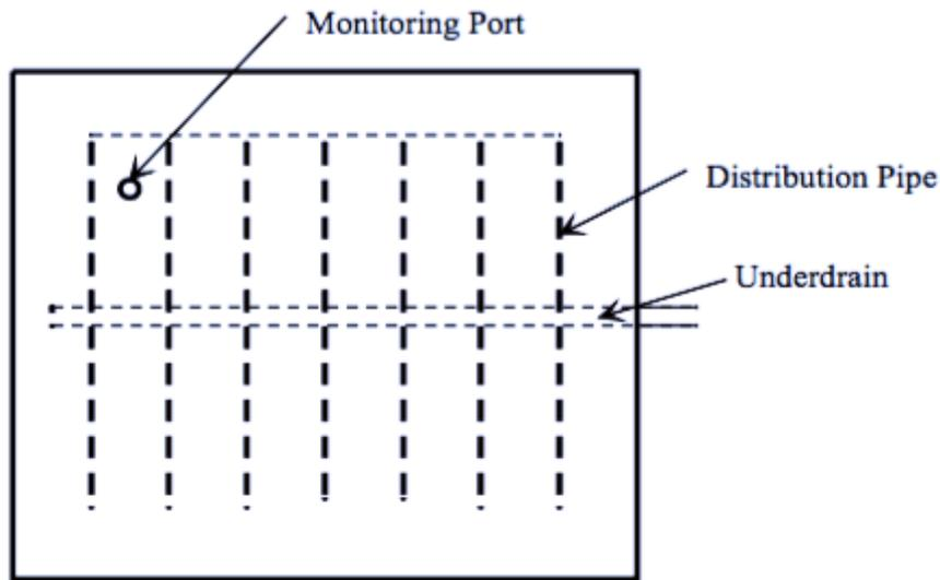
Fig. 2 Typical Intermittent Sand Filter Top View, Washington State Department of Health’s Recommended Standards and Guidance for Intermittent Sand Filters, July, 2012.
