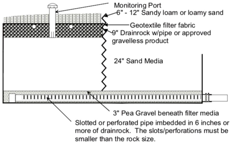
Fig. 1 Typical Intermittent Sand Filter Cross Section, Washington State Department of Health's Recommended Standards and Guidance for Intermittent Sand Filters, July, 2012.
