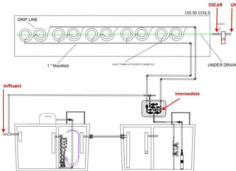
Figure 4, OSCAR-Nitro schematic
