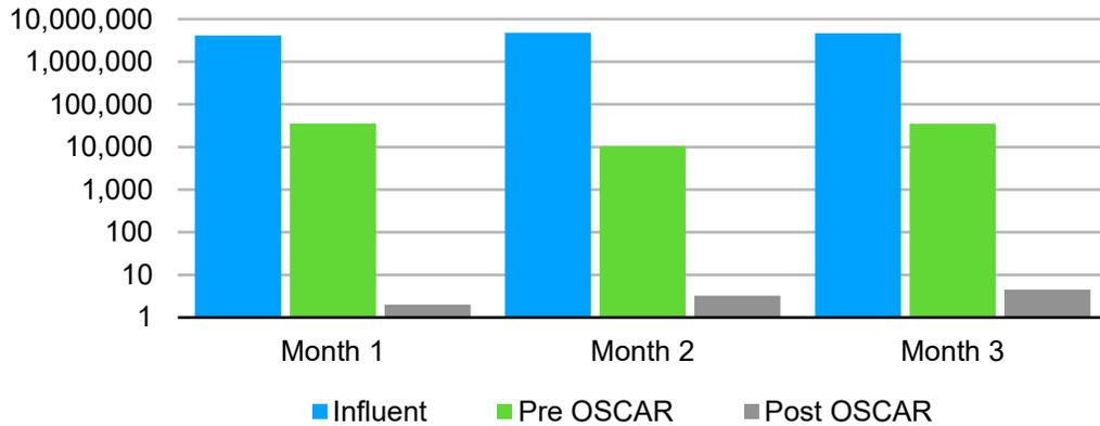
Figure 5, Graph of geometric means of fecal coliform concentration throughout the treatment process.
