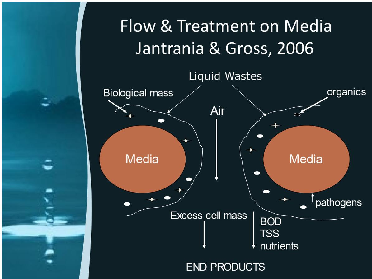
Figure 1. Flow path and treatment areas in a media filter.
