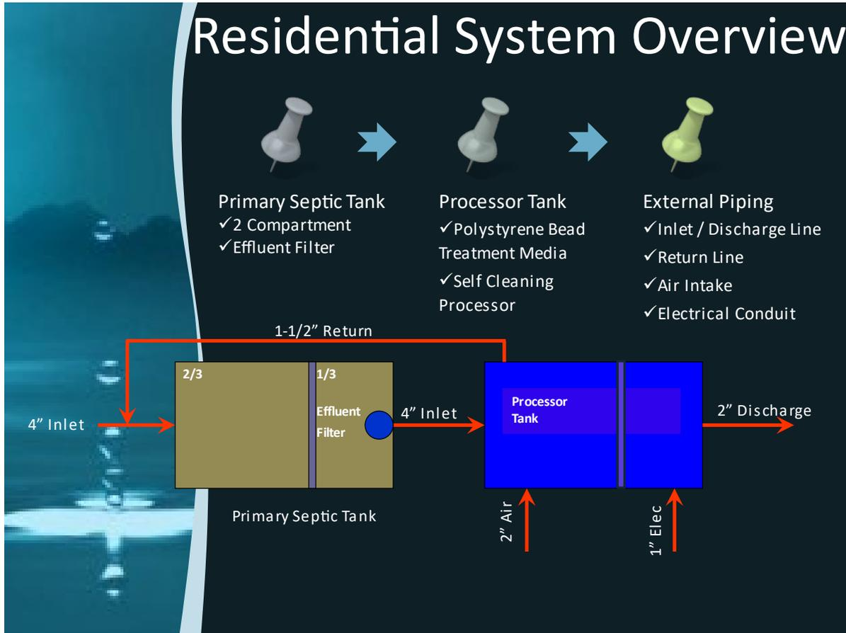
Figure 4. Plan view of typical STARR® two-tank layout.
