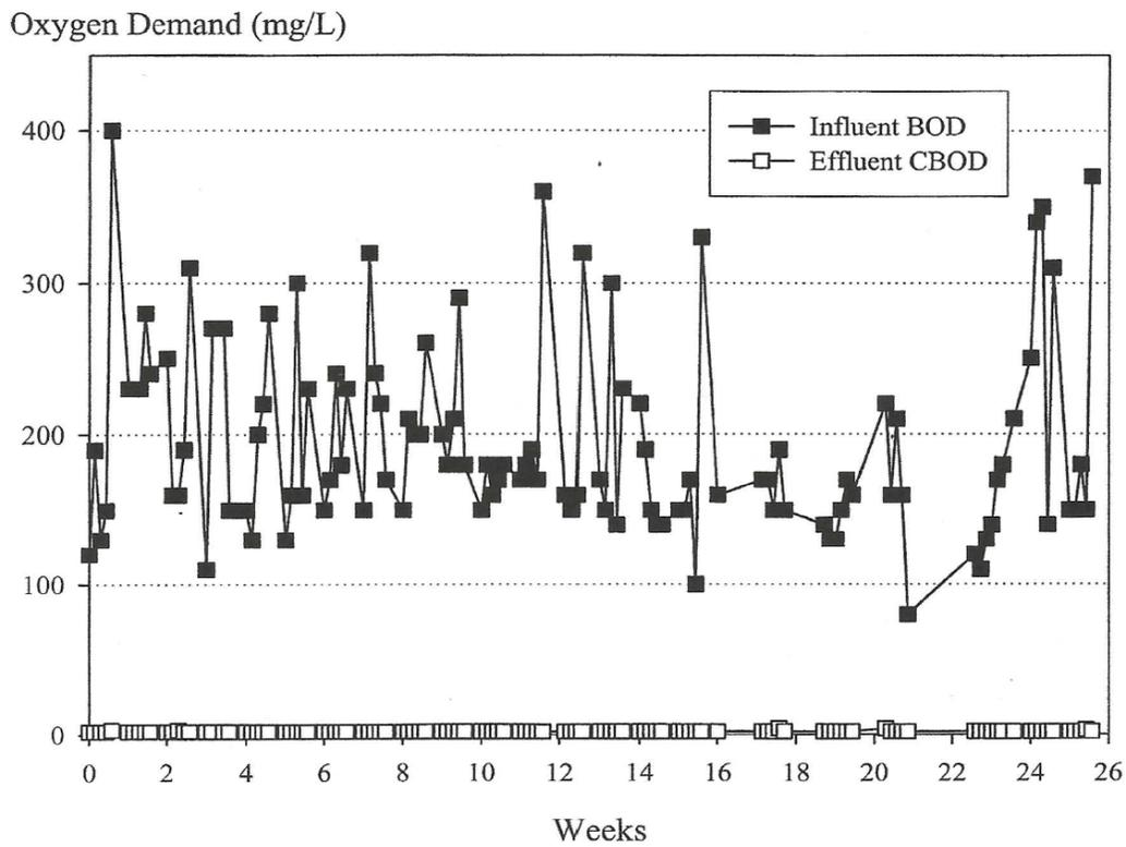
Figure 3. Influent concentrations of 5-day biochemical oxygen demand (BOD<sub>5</sub>) and effluent concentrations of 5-day carbonaceous biochemical oxygen demand (CBOD<sub>5</sub>) during 26-week test period.
