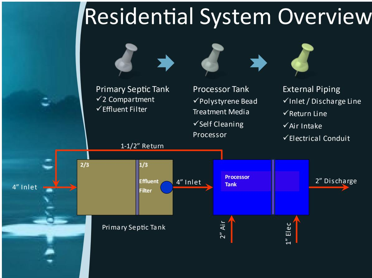
Figure 4. Plan view of typical STARR<sup>®</sup> two-tank layout.
