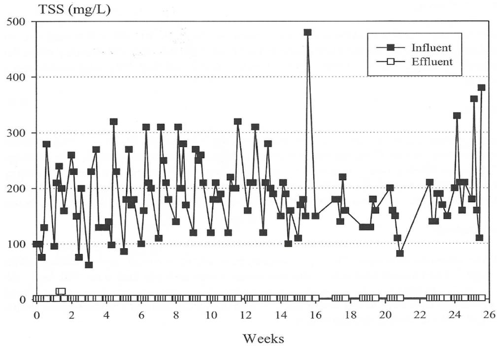
Figure 2. Influent and effluent concentrations of total suspended solids during 26-week test period.
