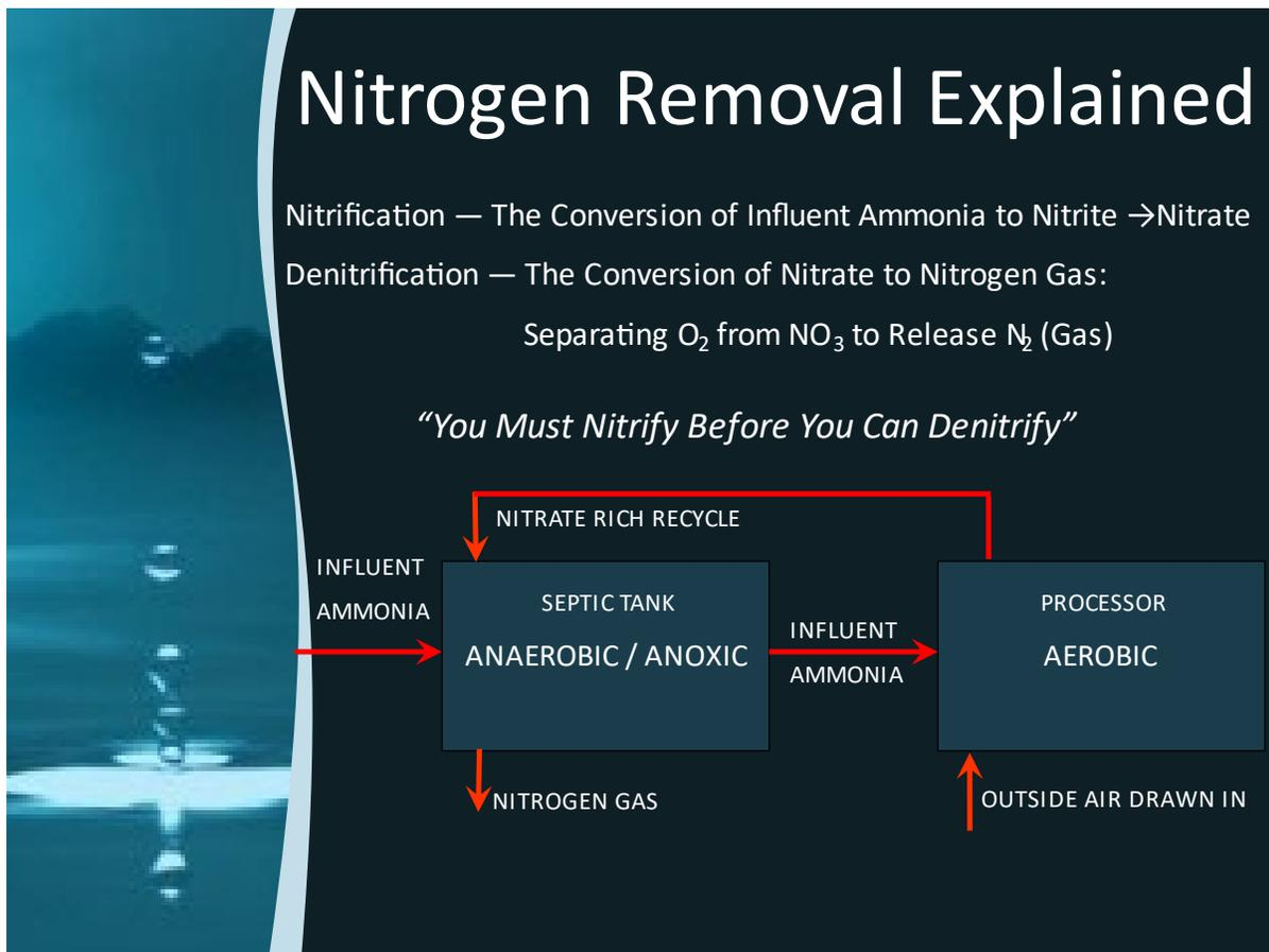
Figure 6. Steps in nitrogen removal with primary nitrogen compound in each location
