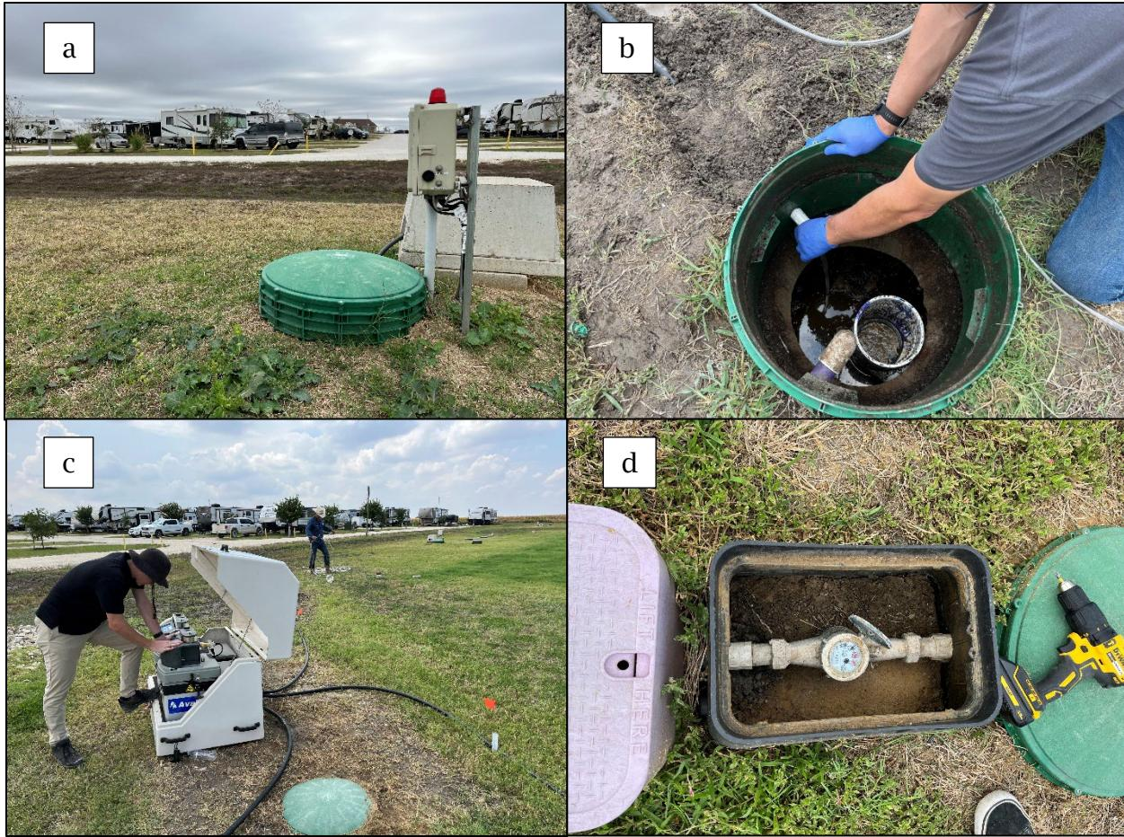
Figure 3. RV park OSSF monitoring configuration: a – Aerobic Treatment Unit with drip system, b – sample intake line installed at wastewater influent point, c – ISCO refrigerated water samplers, d – flow meter.
