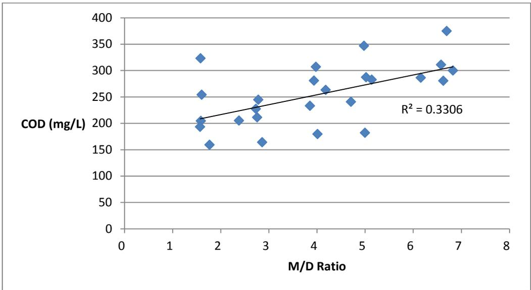
Figure 4-4.  $R^2$  Correlation of M/D Ratio and COD Measurements of Column Effluent of the Final Five Complete Measurements of the First Run (Determining the Effect of Water Softener Usage on Septic Tank Effluent)
