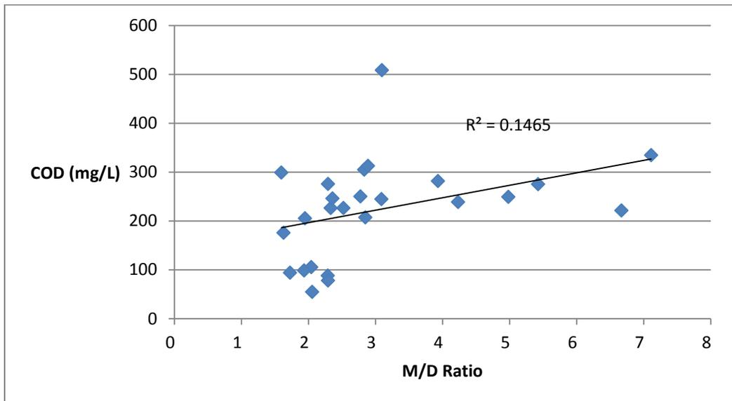
Figure 4-13. R<sup>2</sup> Correlation of M/D Ratio and COD Measurements of Column Effluent of Final Five Complete Measurements of the Second Run (Determining the Effect of Regeneration Wastes on Septic Tank Effluent)
