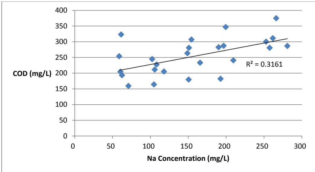
Figure 4-5.  $R^2$  Correlation of Sodium Concentration and COD Measurements of Column Effluent of the Final Five Complete Measurements of the First Run (Determining the Effect of Water Softener Usage on Septic Tank Effluent)
