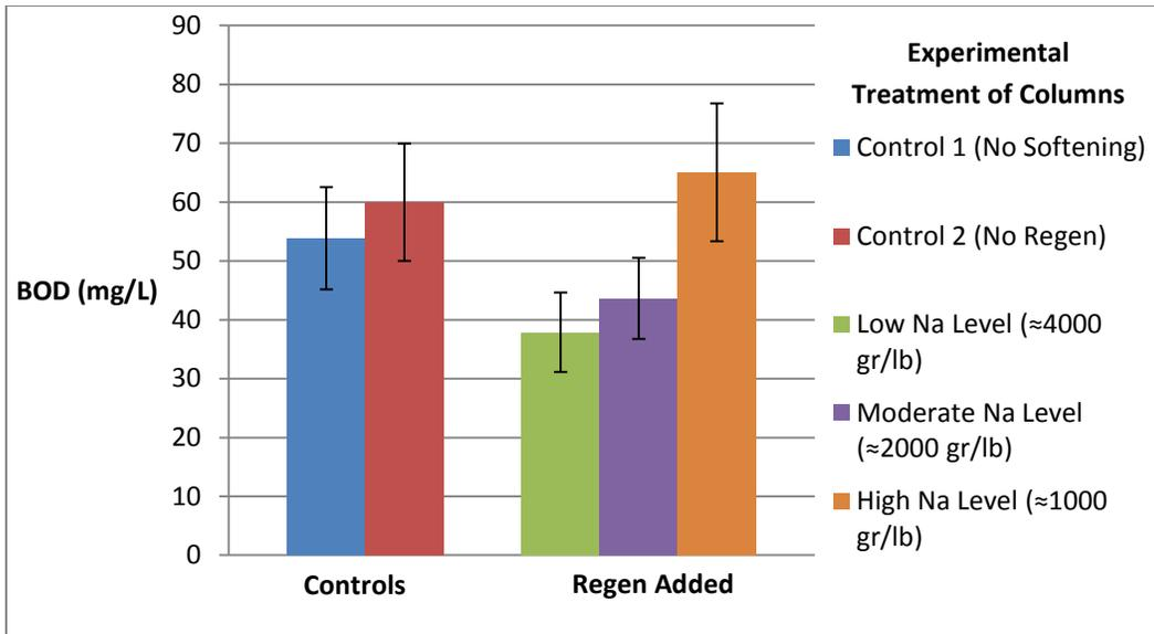
Figure 4-26. Final Five BOD<sub>5</sub> Measurements of Column Effluent During the Fourth Run (Determining the Effect of Regeneration Wastes With Greater Sodium Concentrations on Septic Tank Effluent) Averaged with Standard Deviations
