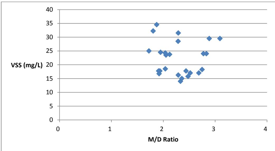
Figure 4-15.  $R^2$  Correlation of M/D Ratio and VSS Measurements of Column Effluent of Final Five Complete Measurements of the Second Run (Determining the Effect of Regeneration Wastes on Septic Tank Effluent)
