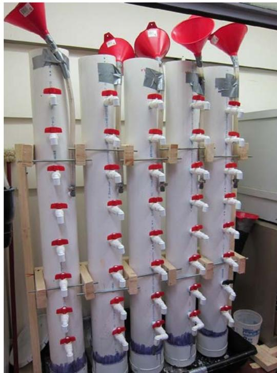
**Figure 3- 1. Column study set up.**
