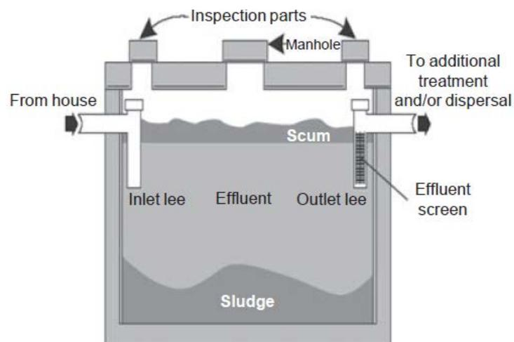
**Figure 2- 3. Typical one compartment septic tank illustrating solids separation and development of clear zone. The outlet tee (on right) is designed to draw clarified effluent from the clear zone, through an effluent screen, and then out of the tank and convey it to the next component (NFSC 2000).**
