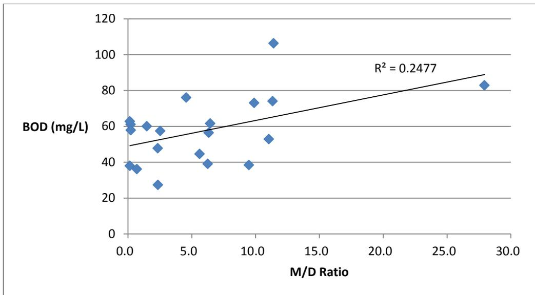
Figure 4-29. Correlation of M/D Ratio and BOD<sub>5</sub> Measurements of Column Effluent of Final Five Complete Measurements of the Fourth Run (Determining the Effect of Regeneration Wastes With Greater Sodium Concentrations on Septic Tank Effluent)
