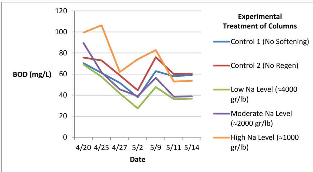
Figure 4-25. Effluent BOD<sub>5</sub> for the Entire Fourth Run (Determining the Effect of Regeneration Wastes With Greater Sodium Concentrations on Septic Tank Effluent)
