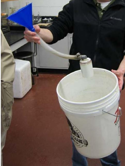
**Figure 3- 2. Effluent screen set up.**
