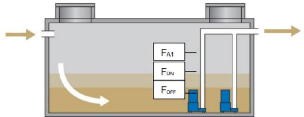
Figure 1: Schematic representation of the position of the floats in the Equalization Tank
