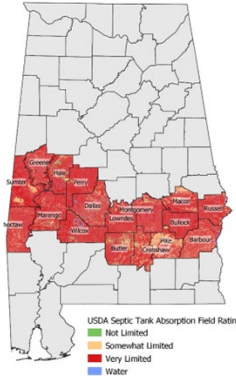
Photo 1. Soil conditions for onsite wastewater treatment systems in the Alabama Black Belt.
