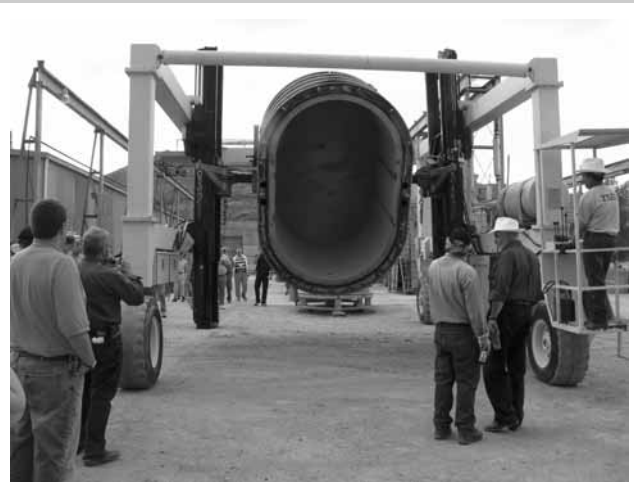
Front Range Precast Concrete president, Doug Jatcko , shows field trip participants the Halo direct control robot that allows a single operator to manipulate forms, strip tanks, move inventory, and load trucks efficiently and safely. This greatly reduces necessary manpower, increases levels of quality assurance and control, and allows precast concrete manufacturers to effectively concentrate on mass production.
