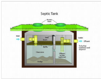
Septic Tank Septic tank, inlet and outlet piping, baffles, sludge and scum accumulation, profile, color
