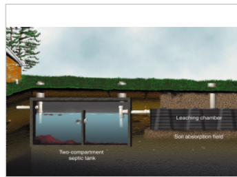
Septic tank and leaching chamber STA
