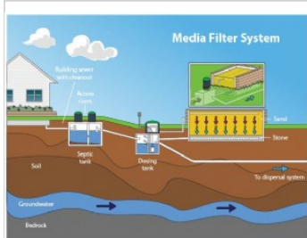
Recirculating media filter system
