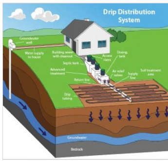
Drip distribution Residential OWTS: gravity septic tank, dosing tank, drip distribution STA, 3D color
