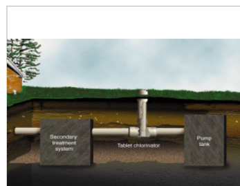
Chlorination unit in a treatment system
