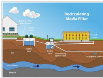
Recirculating media filter, split base Residential OWTS: gravity septic tank, dosing tank, recirculating media filter with split base, recirculating splitter valve, profile view, color
