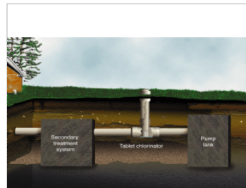
Chlorination unit in a treatment system
