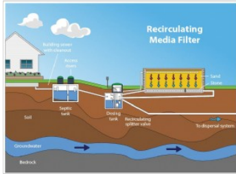
Recirculating media filter, split base
