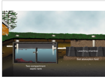
Septic tank and leaching chamber STA
